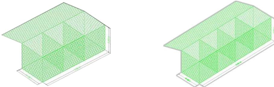
*Figure 7. 3x1x1m and 4x1x1m Gabion Cages from SOLID.PH*
